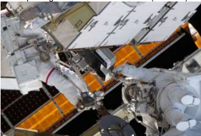
3. Replacing batteries on the P6 truss (© NASA)
