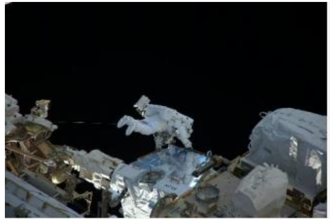
4. An astronaut installing a new-generation battery during a space walk (© JAXA/Roscosmos)
