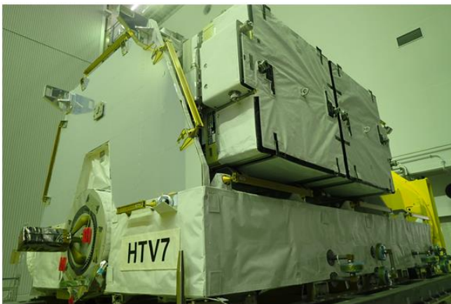
3. Exposed pallet installed with Lithium-ion batteries for ISS to be loaded in "KOUNOTORI" 7 (© JAXA)
