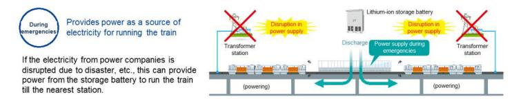
Under normal conditions Regenerative power is stored to provide electricity when needed
