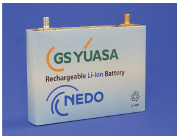
Fig. 1 External appearance of newly developed 11 Ah-class lithium-ion battery with \text{LiNi}_x\text{Mn}_y\text{Co}_z\text{O}_2(x+y+z=1) - \text{LiFePO}_4 composite positive.
