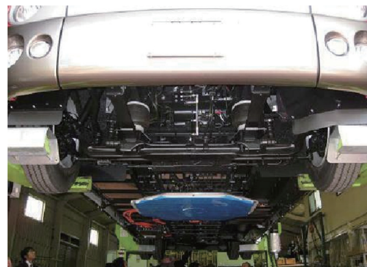
Fig. 5 Latest IPS wireless charging system model: (a) Primary side and (b) Secondary side.
