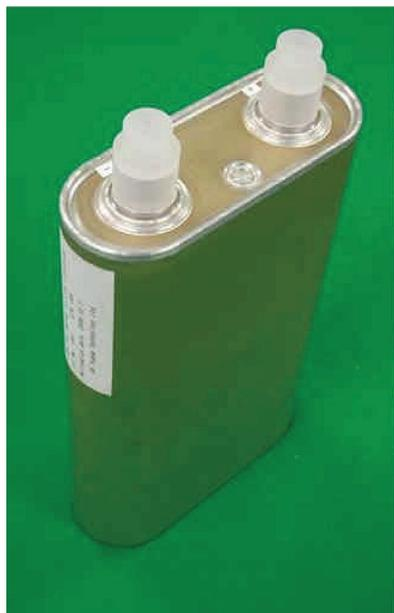
Fig. 3 Appearance of a prototype high energy density lithium-ion cell for lunar exploration mission.
