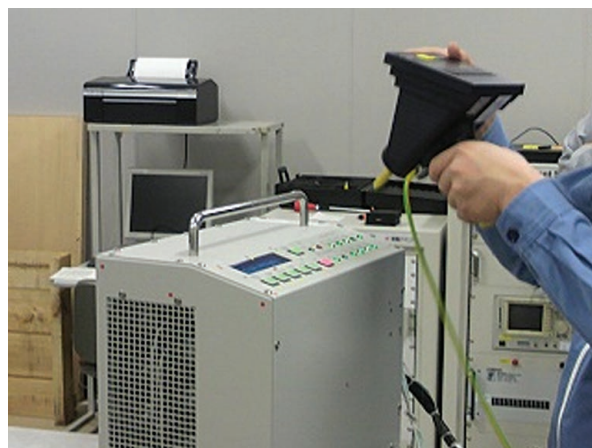
Fig. 9 Experimental scenery of electrostatic discharge in EMC tests for GSE "BH DU3924".
