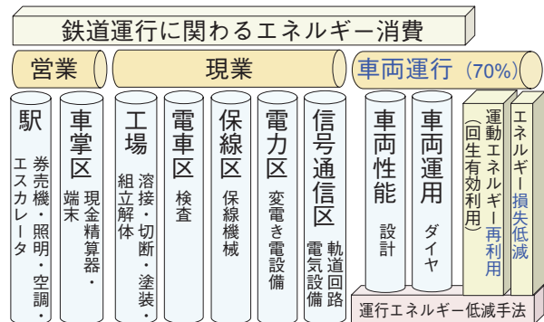
図2 鉄道事業に関わるエネルギー消費 Fig. 2 Energy consumption of rail-operation business.
