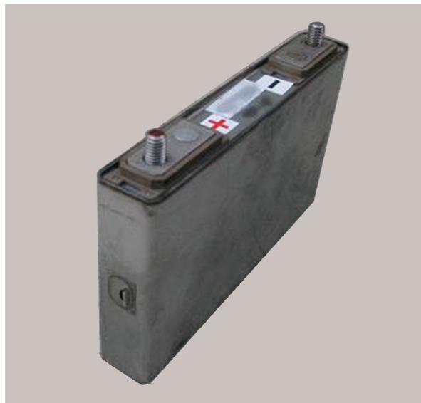
Fig. 13 Outer appearance of prototype 25 Ah  $\text{LiFePO}_4$ /graphite lithium-ion cell after overcharge test.
