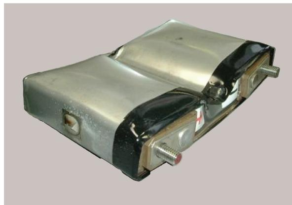
Fig. 11 Outer appearance of prototype 25 Ah LiFePO<sub>4</sub>/graphite lithium-ion cell after crush test.
