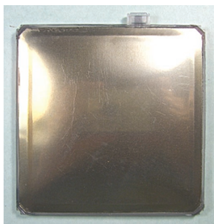
Fig. 4 External appearance of advanced 2 V-1.6 Ah type VRLA experimental cells using Ti/SnO 2 positive current collector.
