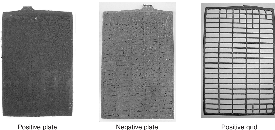
Fig. 6 External appearance of plates for newly developed GYZ20L type VRLA battery after life cycle performance test with high rate discharge. Positive plates shows little change from initial condition. Its corrosion ratio is as little as 7%. Battery came to its life by the shrinkage of negative active material.
