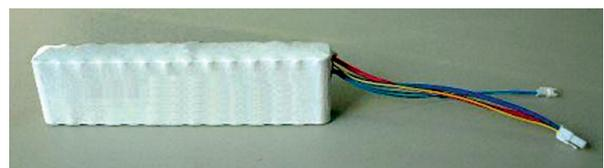
Fig. 3 External appearance of Ni-MH battery pack for Mini UPS "Acrostar THA1000-10-N" of 1 kVA/800 W. Dimensions: 263 mm W x 44 mm D x 72 mm H, Mass 4 kg.
