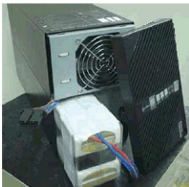
Fig. 2 External appearance of Mini UPS "Acrostar THA1000-10-N" of 1 kVA/800 W. Dimensions: 143 mm W x 395 mm D x 222 mm H, Mass 12 kg.
