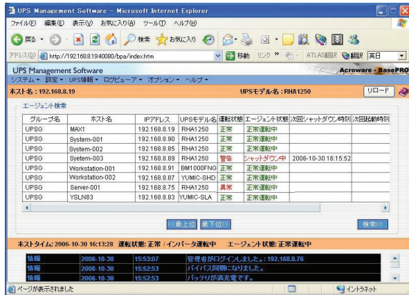
Fig. 3 A display of monitoring screen for searching UPS through web browser of internet.
