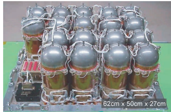
Fig. 2 100 Ah Ni-H 2 assembly for the ETS-VIII. The photograph shows half unit of the battery.
