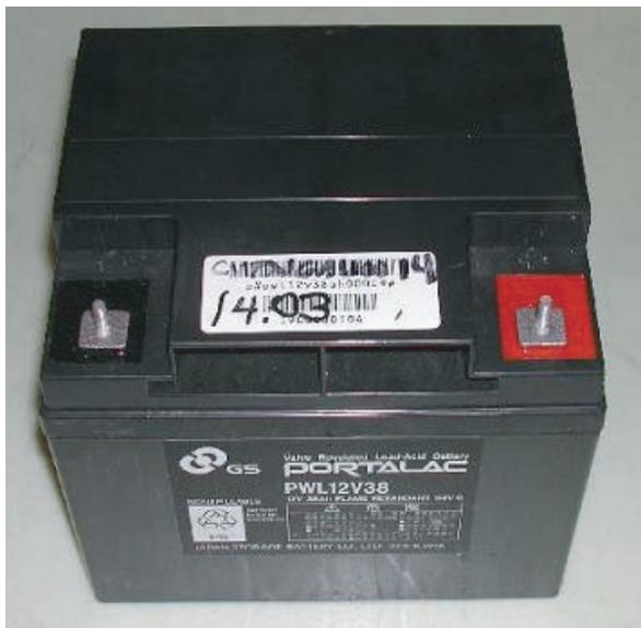
Fig. 8 Outside view of PWL12V38 valve regulated lead acid battery used for about 3 years at outdoor cabinet type C of remote terminal application at Covington, GA (Site No.2).
