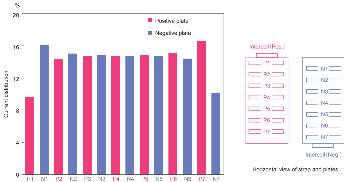
Fig. 6 Computed current distribution to plates during AC-IR measurement. The numbers below the graph and the right figure represent the position of plates.
