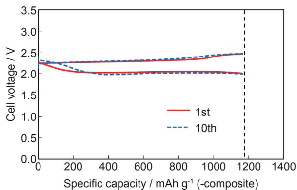
Fig. 9 Charge-discharge performances at 1st and 10th cycles for the Li-S cell with Li-Nafion separator using 0.5 M  $\text{Li}_2\text{S}_6$  in DOL-DME at 25°C. The current is 0.1 CA ( $167.5 \text{ mA g}^{-1}$ -sulfur). The value of capacity limitation is  $1170 \text{ mAh g}^{-1}$  calculated from theoretical capacity of sulfur and its content in SPC.
