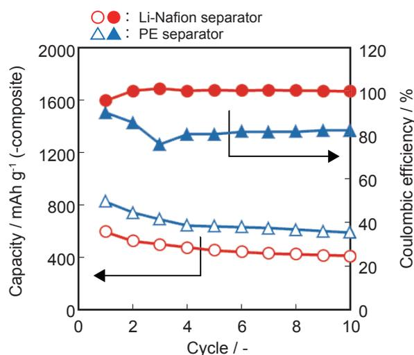
Fig. 4 Changes in discharge capacities and coulombic efficiencies for the Li-S cells with Li-Nafion separator and PE separator using 1.0 M LiTFSI in DOL-DME at 25°C. The current and cutoff voltage are 0.1 C (167.5 mA g<sup>-1</sup>-sulfur) and 1.0–3.0 V, respectively.
