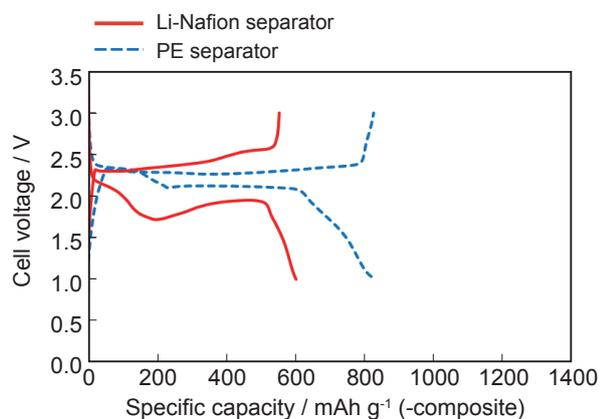
Fig. 3 Charge-discharge performances for the Li-S cells with Li-Nafion separator and PE separator using 1.0 M LiTFSI in DOL-DME at 25°C. The current and cutoff voltage are 0.1 CA (167.5 mA g<sup>-1</sup>-sulfur) and 1.0–3.0 V, respectively.
