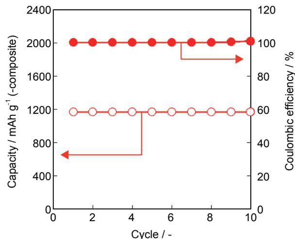
Fig. 10 Changes in discharge capacity and coulombic efficiency for the Li-S cells with Li-Nafion separator using 0.5 M  $\text{Li}_2\text{S}_6$  in DOL-DME at 25°C. The current is 0.1 CA ( $167.5 \text{ mA g}^{-1}$ -sulfur). The value of capacity limitation is  $1170 \text{ mAh g}^{-1}$  calculated from theoretical capacity of sulfur and its content in SPC.
