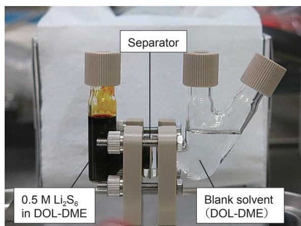
Fig. 1 Setup of the glass cell for the measurement of polysulfide permeation.
