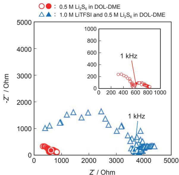
Fig. 8 Cole-Cole plots of the Li-S cells with Li-Nafion separator using 0.5 M  $\text{Li}_2\text{S}_6$  or the mixed solution of 1.0 M LiTFSI and 0.5 M  $\text{Li}_2\text{S}_6$  in DOL-DME at 25°C.
