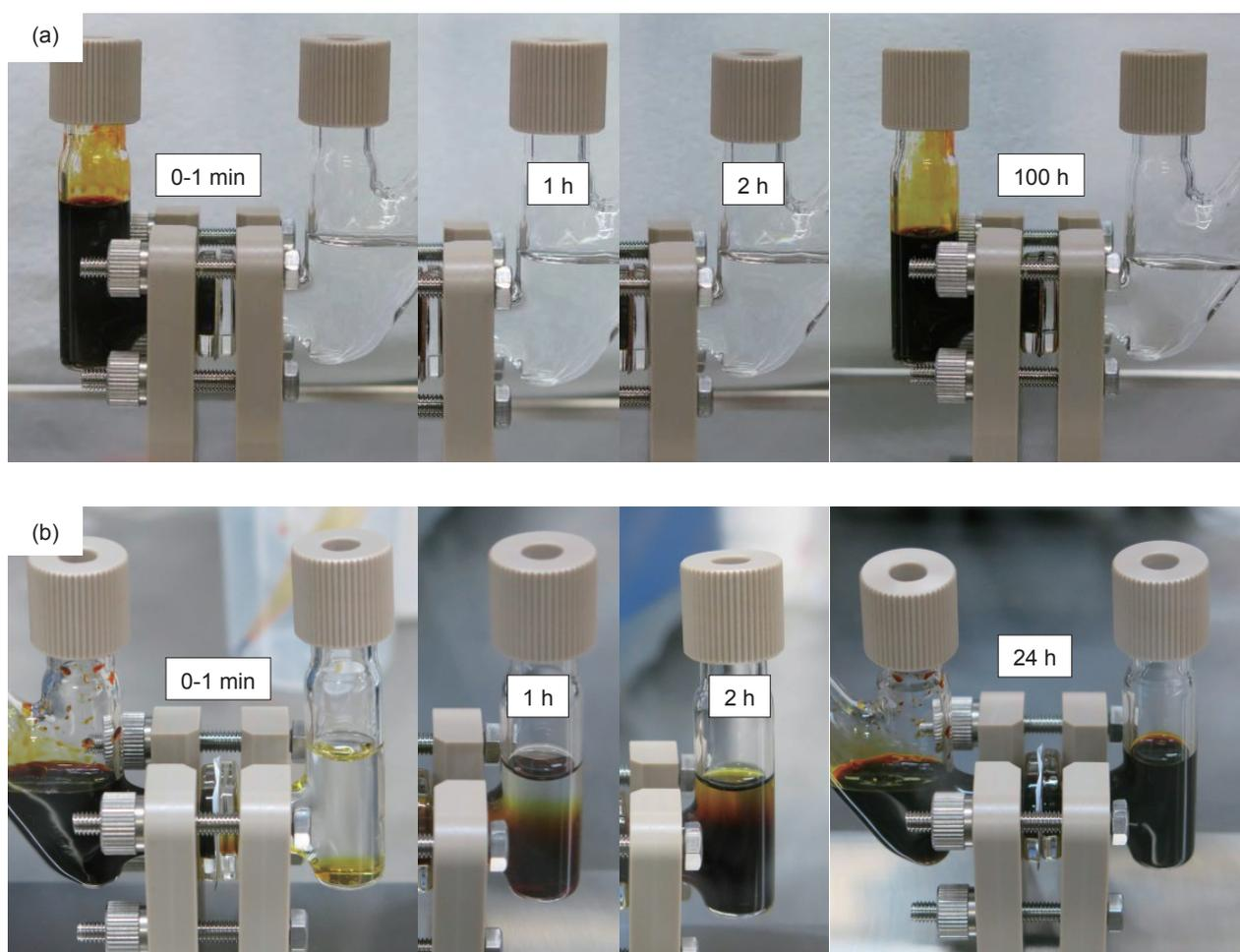
Fig. 2 Comparison of polysulfide permeation through (a) Li–Nafion separator swollen by DOL–DME solvent and (b) conventional polyethylene separator.
