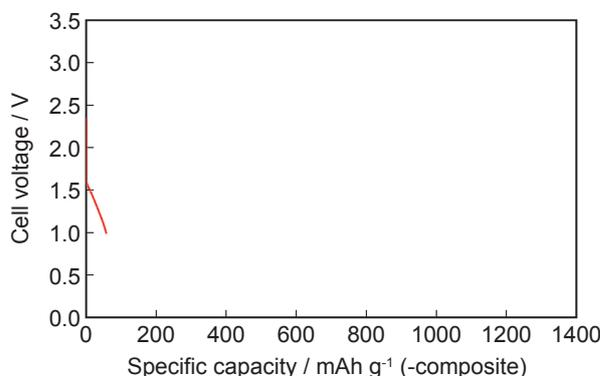
Fig. 5 Discharge performance for the Li-S cell with Li-Nafion separator using the mixed solution of 1.0 M LiTFSI and 0.5 M Li<sub>2</sub>S<sub>6</sub> in DOL-DME at 25°C. The current and cutoff voltage are 0.1 CA (167.5 mA g<sup>-1</sup>-sulfur) and 1.0 V, respectively.
