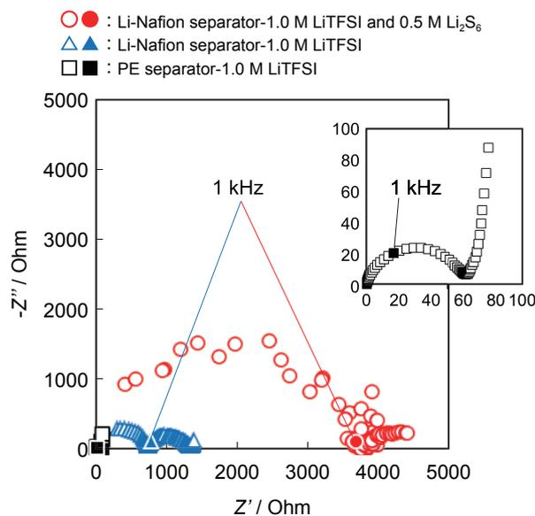
Fig. 6 Cole-Cole plots of Li-S cells with the Li-Nafion separator using the mixed solution of 1.0 M LiTFSI and 0.5 M Li<sub>2</sub>S<sub>6</sub> or 1.0 M LiTFSI and PE separator using 1.0 M LiTFSI in DOL-DME at 25°C.
