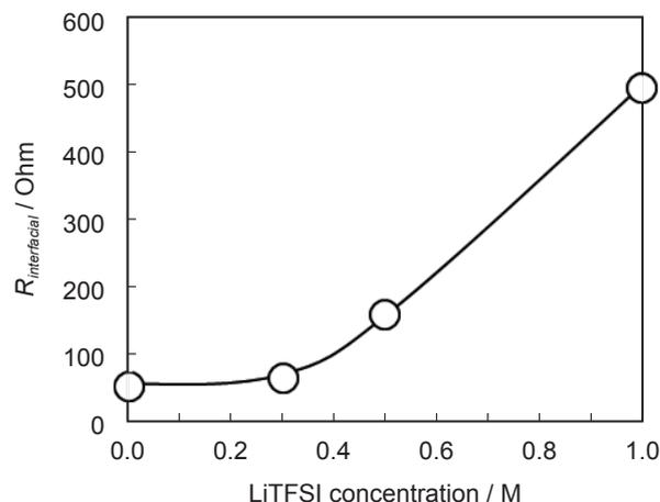
Fig. 7 Influence of LiTFSI concentration in the mixed solution containing 0.5 M Li<sub>2</sub>S<sub>6</sub> in DOL-DME on interfacial resistance between the solution and Li-Nafion separator at 25°C.
