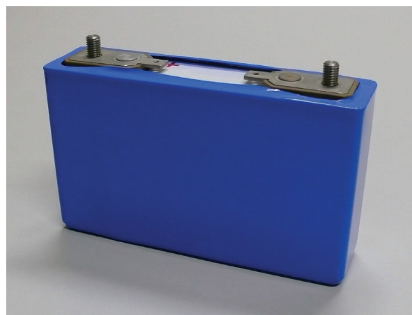
Fig. 1 Appearance of prototype 50 Ah \text{LiFePO}_4/\text{graphite} lithium-ion cell.
