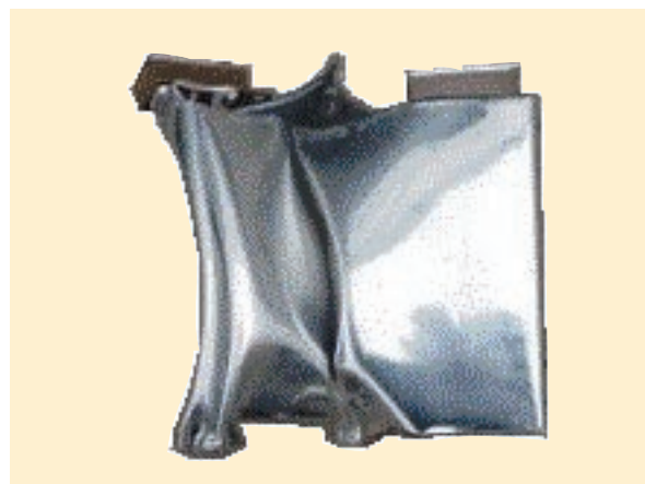
Fig. 13 Outer appearance of newly developed 20 Ah LiFePO 4 /graphite lithium-ion cell after crush test in Y-axis direction.
