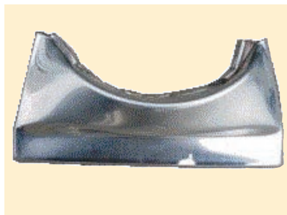
Fig. 14 Outer appearance of newly developed 20 Ah LiFePO 4 /graphite lithium-ion cell after crush test in Z-axis direction.
