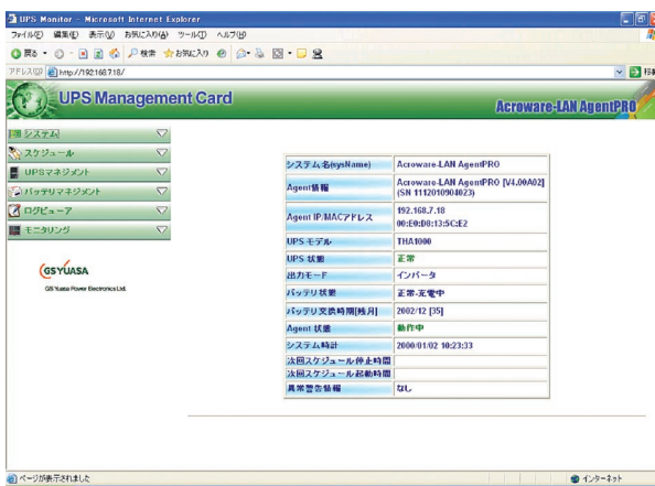
Fig. 2 External appearance and monitor image of network interface "Acroware-LAN AgentPRO".
