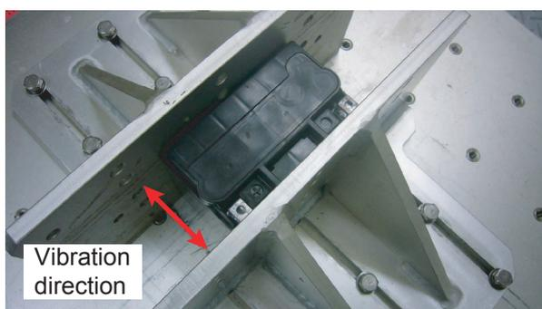
(b) Vibrating towards short side direction parallel to the plate surface
