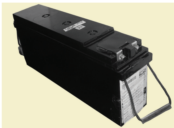
Fig. 3 Outside view of PWL12V100FT valve regulated lead-acid battery used for 4.2 years at outdoor cabinet for telecommunication utility in Athens, GA.
