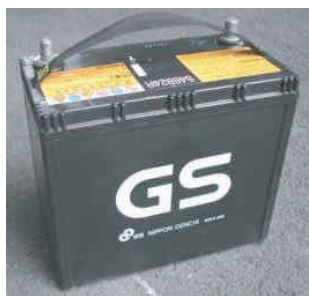
Fig. 4 Photograph of VRLA battery for auxiliary equipment in hybrid vehicle "Prius".
