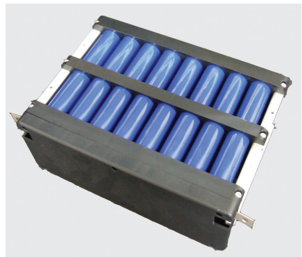
Fig. 5 External appearance of 0.3 kWh-class prototype lithium-ion battery module.
