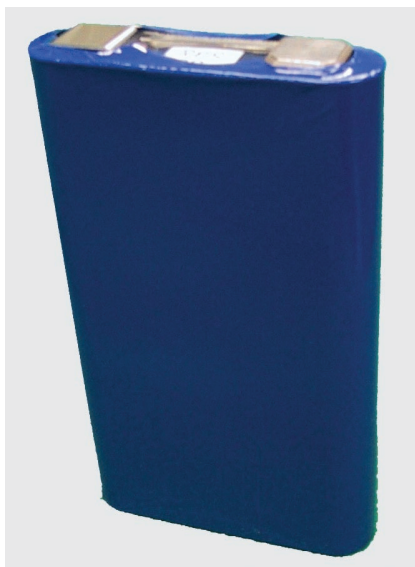
Fig. 4 External appearance of 10 Ah-class prototype lithium-ion single cell with ellipse-shape case.
