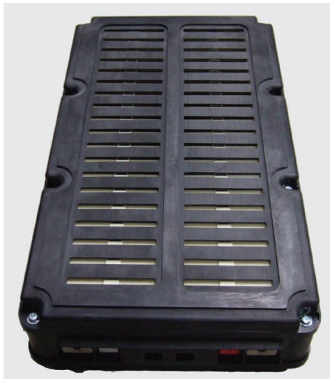
Fig. 3 External appearance of 1 kWh-class prototype lithium-ion battery pack with new arrangement of single cells for uniformity air-cooling system.
