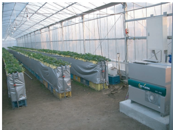
Fig. 4 Scenery of 1 kW class DMFC system applied to the agriculture field test.
