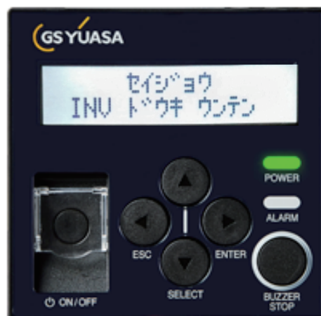
図2 操作表示部の拡大写真 Fig.2 Enlarged image of the LCD and switch unit.
