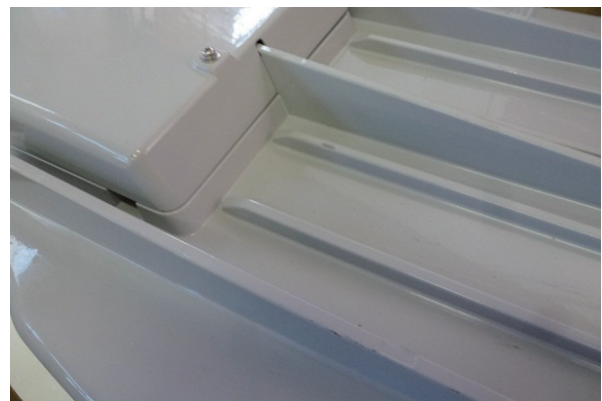
Fig. 8 The ribs on the roof of envelope for thermal evacuation.
