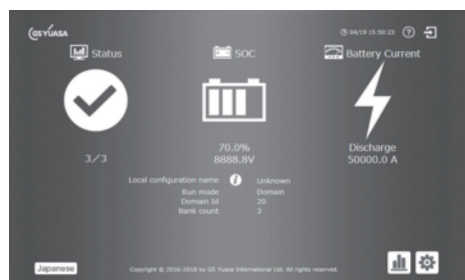
●Fig. 2 Web interface presented by the remote monitoring system server
