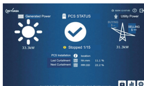
●Fig. 3 Web interface presented by a communication device attached to a power conditioner (PCS)
