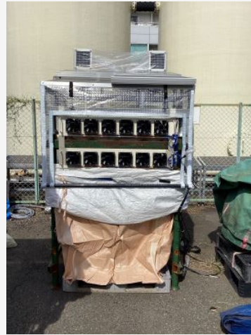
Dewatered sludge dryer
