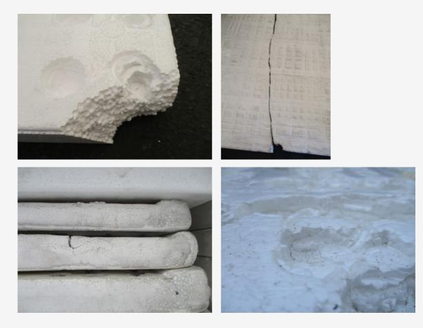
Use limited samples of Styrofoam (top row: chipping, cracking; bottom row: insufficient thickness, water dripping)
